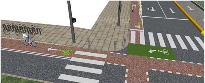
Concept drawing of an unprotected intersection.
