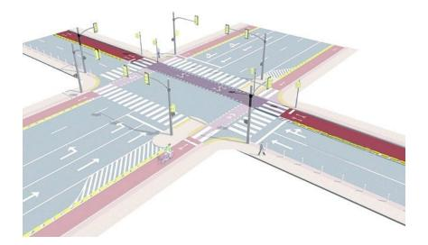
*Bi-directional protected lanes separated from car traffic through physical barrier.*
