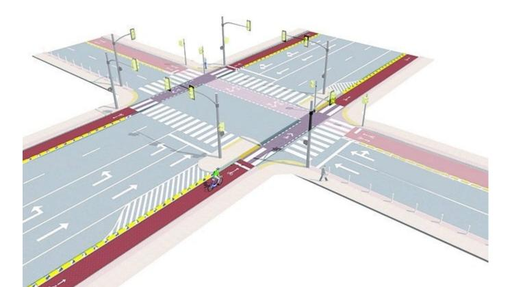
Uni-directional protected lanes separated from car traffic through physical barrier. Graphic by WRI.
